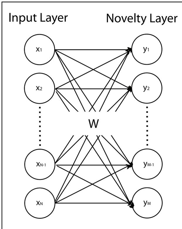
**Figure 14. The Infomax model.** Circles represent units and arrows denote connections between the input units on the left and the novelty units on the right. There is no output from the network as such since the response of the network is a function of novelty unit activations. Following [59] we therefore do not draw an output layer. doi:10.1371/journal.pcbi.1002336.g014
