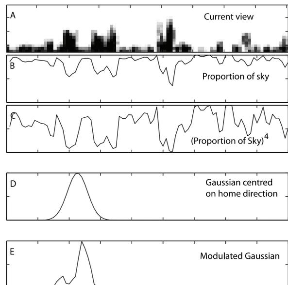
**Figure 11. Path integration modulated by obstacle avoidance.** A,B,C) Obstacle avoidance is achieved by biasing movements towards low points on the horizon. D) A Gaussian distribution is centred on the home direction. E) The Gaussian is multiplied by the proportion of sky raised to the power of 4 and then normalised. This distribution is then sampled from to determine a movement direction.
