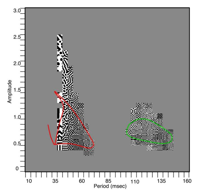
Figure 6. Two-parameter phase diagram for the model. Each square is a simulation of a  $64 \times 64$  domain with periodic boundary conditions. Patterns are shown as the period and amplitude range over the relevant intervals. Colored curves represent the theoretical boundaries for instability of the spatially uniform state. doi:10.1371/journal.pcbi.1002158.g006
