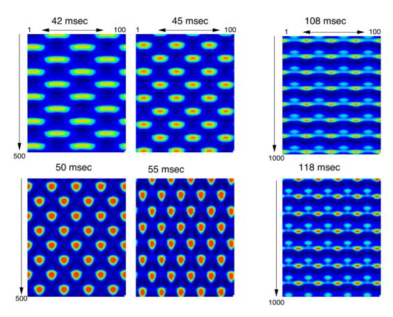
Figure 2. Space-time evolution of patterns produced by equations (1,2) in a one-dimensional spatial domain.  $\sigma_e = 2, \sigma_i = 5$ , with periodic boundary conditions. Time increases in the vertical direction. Amplitude of the stimulus was 0.8 and the period of the stimulus is shown above each panel. doi:10.1371/iournal.pcbi.1002158.g002
