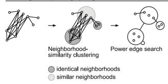
**Figure 12. Power graph algorithm.** First a neighbourhood similarity clustering of the nodes is performed providing candidate power nodes. In a second step power edges are searched between nodes and candidate power nodes. Note that modular decomposition would not consider as a module the set of nodes having similar but non-identical neighbourhoods. The power graph algorithm finds this candidate and uses it to succinctly represent the biclique. doi:10.1371/journal.pcbi.1000108.g012
