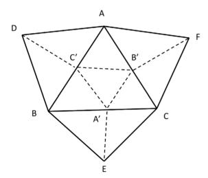
**Figure 1. Mesh refinement procedure.** When the area of a triangle ABC exceeds two times the averaged area of the triangles of the original mesh we divide the original triangle in four triangles constructed from the three midpoints  $A'_{,B',C'}$  of each side. Moreover we divide each of the three triangles ABD, ACF, BCE in two triangles. doi:10.1371/journal.pcbi.1000749.g001
