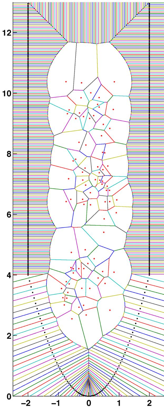
**Figure 4. Typical initial configuration of cells after the Voronoi tessellation of random generating points.**
